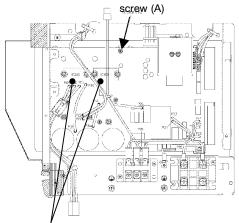
Apply thermal grease to <u>the back</u> (heat sink contacting side) of IC200 and IC300.
